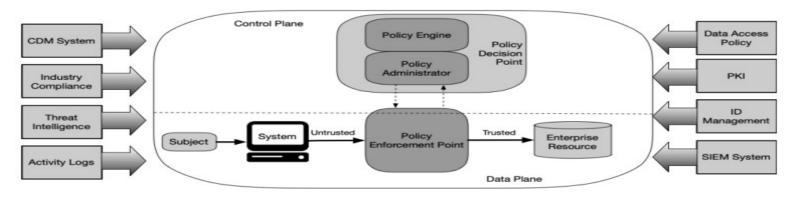
PDP consist of PE and PA and uses the Control Plane for communications between the two
